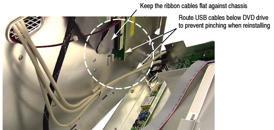
Figure 5-5: Dress the cables properly
